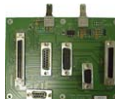
T21 Junction Board
